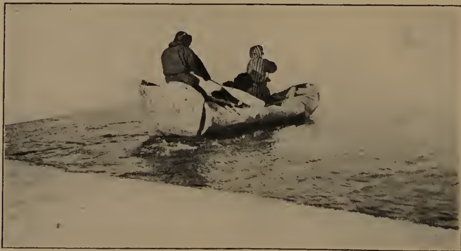
CROSSING LEAD IN SLED RAFT MADE BY STRETCHING WATERPROOFED CANVAS ABOUT SLED AND LASHING IT TO SIDES.
